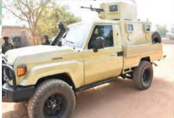
DAY TESTING OF VANQUISHER APC 360 DEGREE ROTATING TURRET
