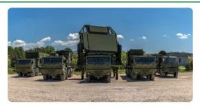
ALP 300-G, is a new generation S-Band radar developed for long range early warning, with its AESA and digital beamforming antenna architecture. ALP 300-G has the ability to detect and track air breathing targets, ballistic missiles, anti-radiation missiles and stealth/low RCS targets from very long ranges.
